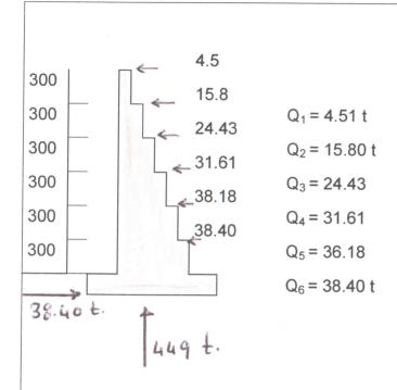
Sectional allocation for the floor columns
